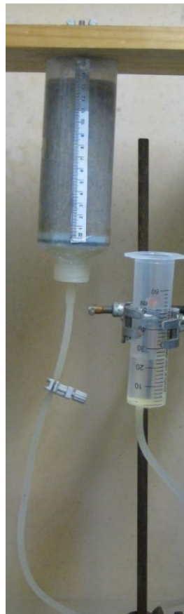
Fig 3.1 Sediment filled columns were held suspended to a wooden board for the drawdown experiments
